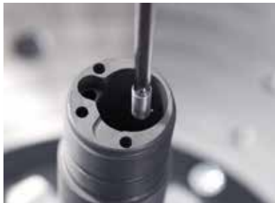
Form measurement in small, deep bores
