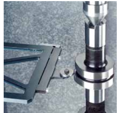
Round measuring follower for camshafts
