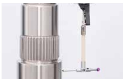
Measurement of roughness and form with double-tipped probe system
