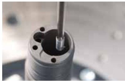
Form measurement in deep, narrow bores
