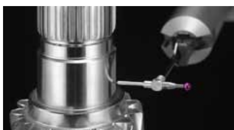
Twist measurement with a roughness stylus tip
