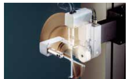
Motorized tilt and rotation module MDS for fully automatic measurement runs (option)
