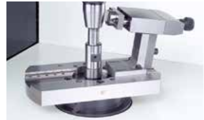
Workpiece-specific radial driver for cam shafts for angle indexing in grooves
