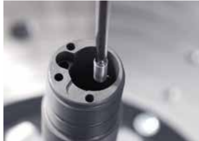
Form measurement in small, deep bores
