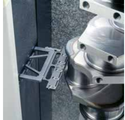
Flat measuring follower for crankshafts
