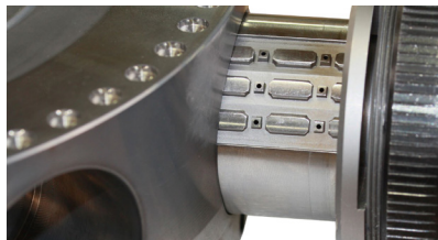
Special air spindle with 12 nozzles for measurement of hydraulic distributor bores
