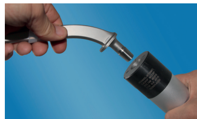
Special air ring for measurement of hip prosthesis
