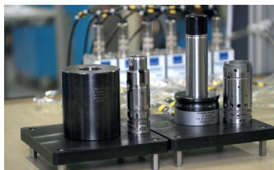
Air ring and air spindle with multiple planes for matching
