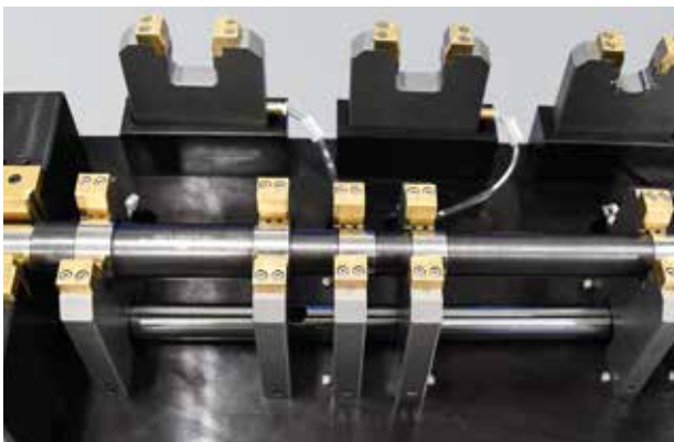
Adjustable fixture using air snap gages
