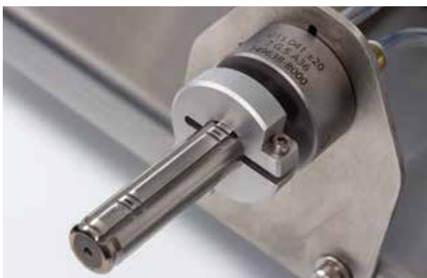
Air spindle with two elongated jets
