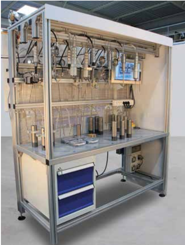
Manual measuring station for cylinder heads
