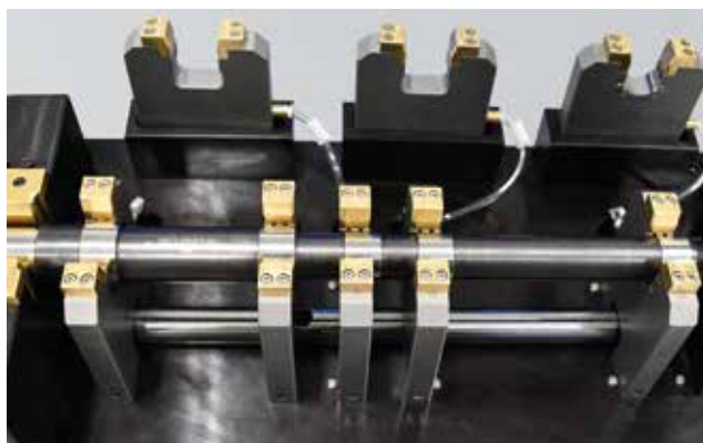
Adjustable fixture using air snap gages
