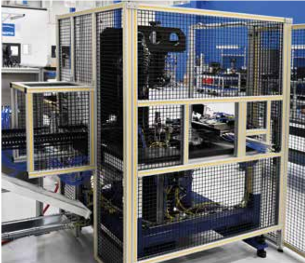
Automatic bench gage for transmission shafts
