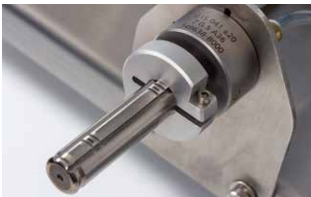
Air spindle with two elongated jets
