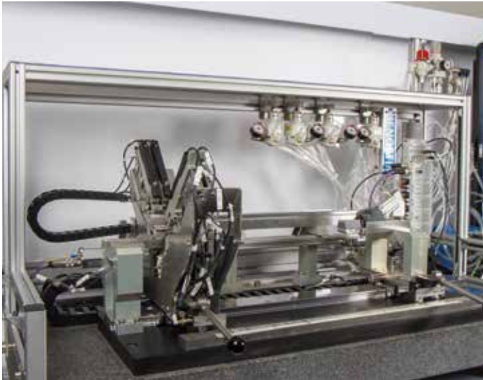
Semi-automatic measuring station for seat rails
