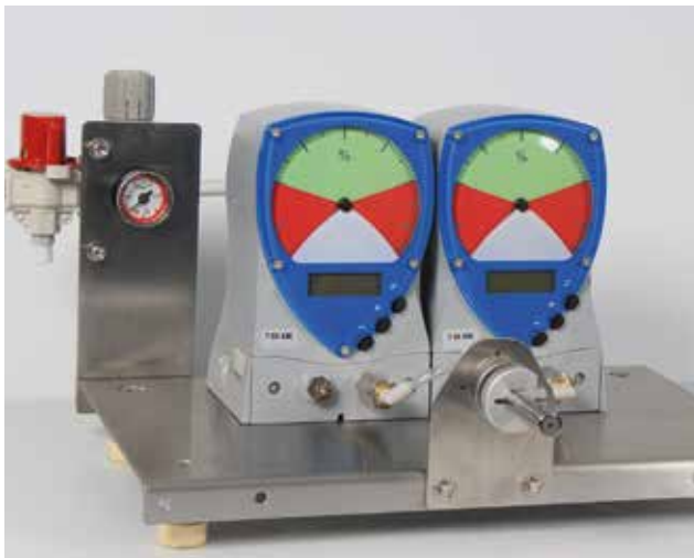
Manual table-top gage for inner diameters
