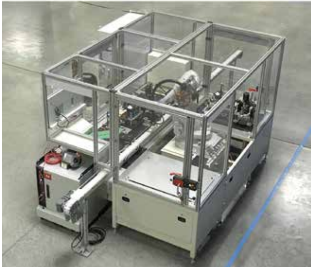
Automated in-line measuring station for gears
