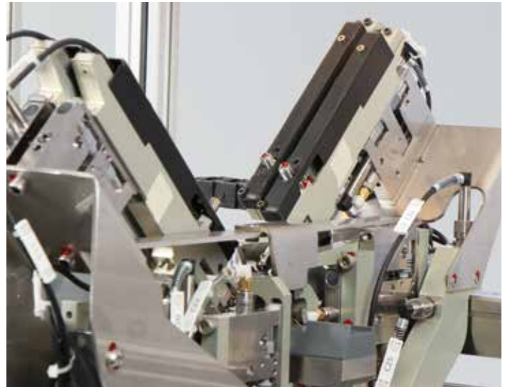
Part-specific tactile measurement
