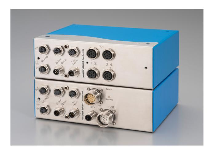
The individual probe satellites of the Gageline PS series can be combined with one another as required and offer various connections.
