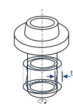
limited by two coaxial cylinders at a distance t apart, the axes of which match the datum axis. After several rotations around the datum axis and axial shift of the transducer all points of the toleranced element must be within the tolerance zone.
