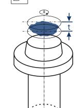
The tolerance zone is limited by two parallel planes at a distance t apart, which are perpendicular to the datum (rotational) axis. After several rotations around the datum axis and radial shift of the transducer, all points of the surface of the tolerance plane face must be within the tolerance zone.
