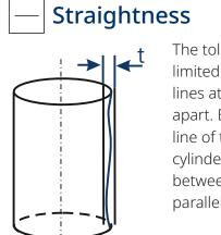
lines at a distance t apart. Every envelope line of the toleranced cylinder must be between these two parallel lines.
