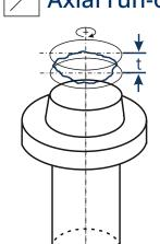
distance of two circles at a distance *t* apart. The circles are in a cylinder, the axis of which matches the datum axis. The diameter of the cylinder can adopt any value of the diameter of the plane face.
