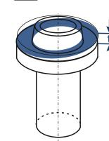
planes at a distance t apart, which are perpendicular The toleranced plane face must be between these two planes.
