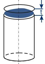
limited by two parallel apart, the dimensions of which correspond to those of the toleranced area. The real workpiece area must be between the two parallel planes at distance *t* apart.
