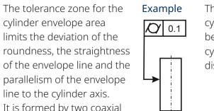
The toleranced cylindrical area must oe between two coaxial cylinders with a radial
