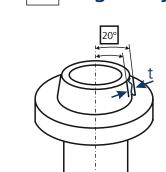
The tolerance zone is limited by two parallel planes at a distance *t* apart at the nominal angle to the datum axis.
