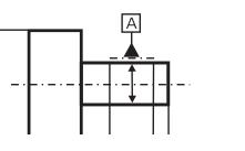
as an extension of the dimension line: if the datum is the axis, the median plane or an appropriately dimensioned point.
