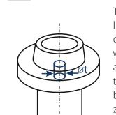
The tolerance zone is limited by a cylinder of diameter t, the axis of which matches the datum axis. The actual axis of the coleranced element must be within the tolerance
