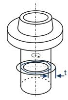
In every radial section plane perpendicular to the surface, the tolerance zone cylindrical area must be circles at a distance **t** apart, between two concentric the common center point circles at a distance apart of which is on the datum of 0.1 with their common center point on the tolerance applies generally for a full revolution of the toleranced element around the datum axis.
