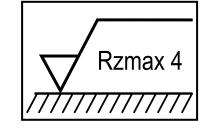
Material removing machining; Rz = max. 4 µm; the maximum value rule applies
