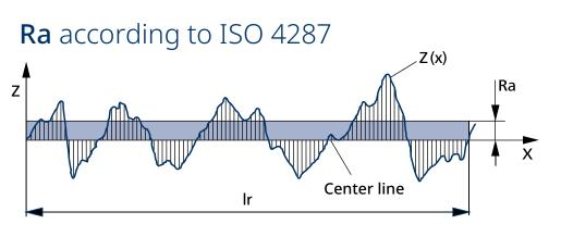
Ra – arithmetical mean deviation Ra is the arithmetic mean roughness value from the amounts of all profile values. Ra does not differentiate between peaks and valleys and has therefore a relatively weak information character.
