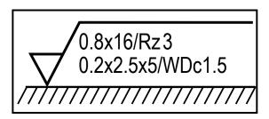
Material removing machining; Rz: the evaluation length is 12.8 mm and  $\lambda c = 0.8$  mm, Rz = max. 3  $\mu$ m; WDc: in the period range of 0.2 to 2.5 mm, WDc = max. 1.5  $\mu$ m applies
