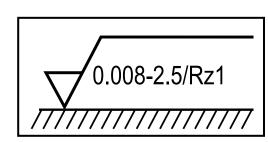
Material removing machining; transmission characteristic does not comply with standarc case (cf. table) Rz = max. 1 μm; filter selection  $\lambda s = 0.008$  mm and  $\lambda c = 2.5$  m
