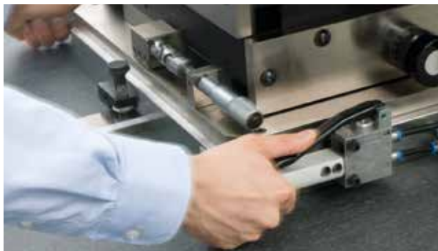
Guided X-Y positioning via air slide with additional fine adjustment
