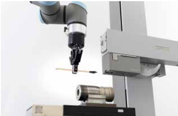
Probe arm change via robot – magnetic holder
