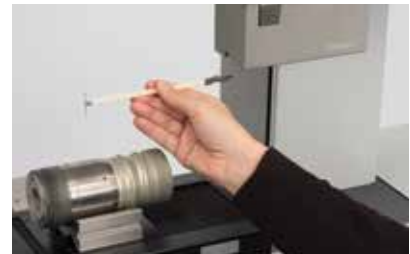
Probe arms with magnetic coupling
