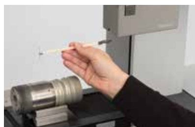
Probe arms with magnetic coupling
