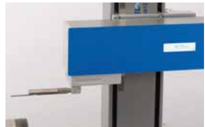
Roughness probe system with quick-change-adaptor
