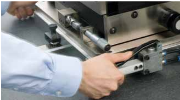
Guided X-Y positioning via air slide with additional fine adjustment
