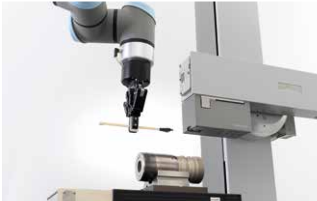
Probe arm change via robot – magnetic holder
