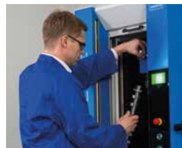
Simple operation of the measuring machine thanks to fast tailstock adjustment
