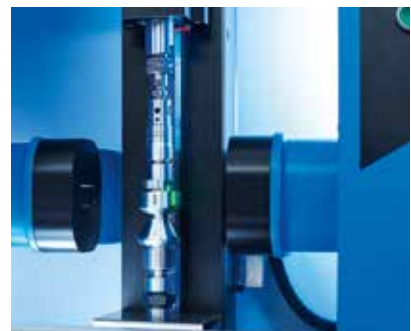
Simple clamping of the workpiece between tips
