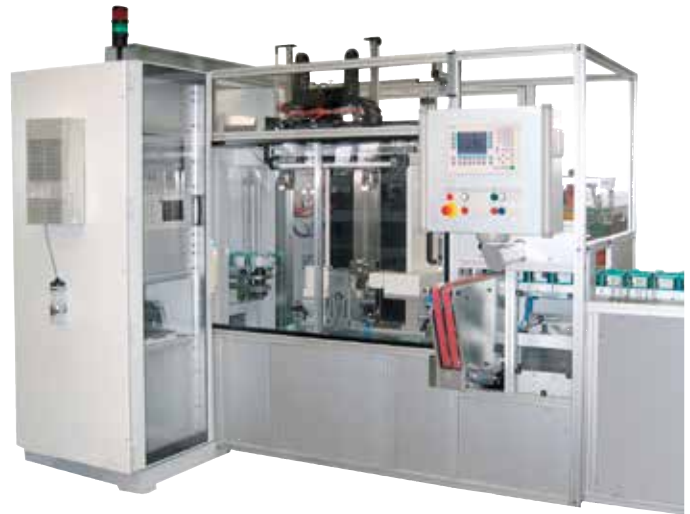
Opticline VMS305 for measuring engine valves; integrated in a production line
