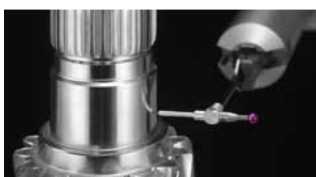
Twist measurement with a roughness stylus tip
