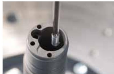
Form measurement in deep, narrow bores
