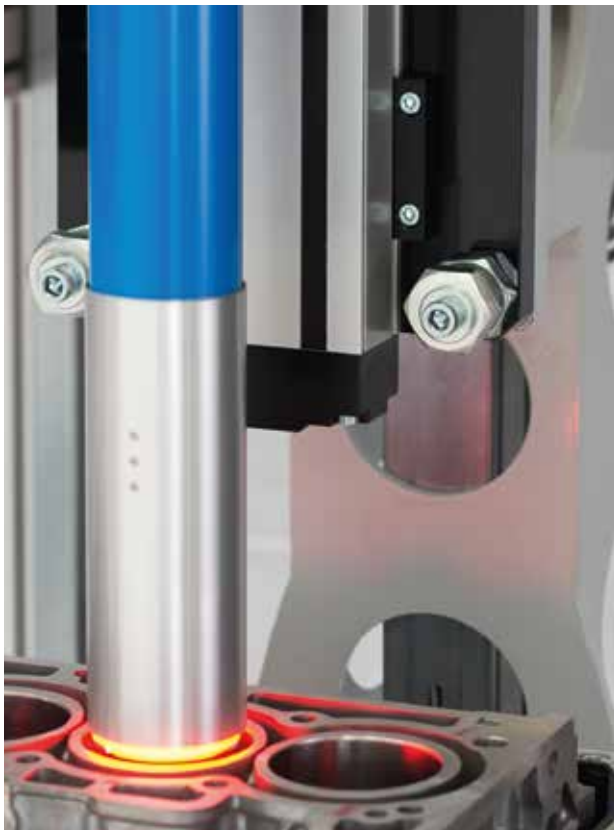
Optical surface inspection in bores
